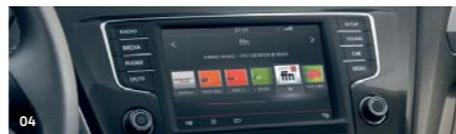
04 The “Composition Media” radio system includes a 20.3 cm (8 inch) TFT colour display, a touchscreen with proximity sensor, and an MP3 and WMA-compatible CD player. Eight loudspeakers with 4 x 20 watts power output transforms every journey into a multimedia experience. Furthermore, the system also features an SD card slot, an AUX-IN jack, a USB port and a Bluetooth connection for mobile telephones.
