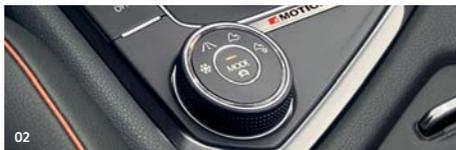
**02** Prepared for everything: the 4MOTION Active Control allows you to choose from four custom designed driving profiles for on-road and off-road driving and an array of different weather situations. 4MOTION Active Control is part of the 4MOTION all-wheel drive.
