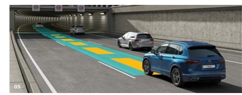
01 The 'ACC' adaptive cruise control adapts the vehicle's speed to that of the vehicle driving ahead up to the maximum speed selected, and maintains the distance set by the driver. (available in KSA only)
